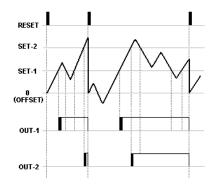
When count value rise from the SET-1, value OUT-1 gives an output and if it rise up from SET-2 value OUT-2 gives an output. Even it falls from the SET value ,relays do not stop until the RESET come, but when the RESET come it stops. If the time is entered for the outputs,relays gives an output and stop during this time,relays do not gives output until the RESET comes, even the fall or rise from the SET values.
