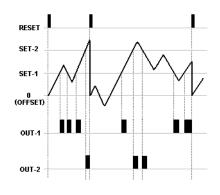
The outputs (TOUT) should be selected as a time in this mode. When the count value's each passing from the SET-1 value, OUT-1 gives an output in TOUT-1 time and stop, each passing the SET-2 value,OUT-2 gives an output and end of the TOUT-2 time it stop. When RESET comes,outputs and count value are reset.
