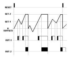
OUT-1 output dependent on OUT-2. TOUT-2 should be selected with time. OUT-1 gives an output, the count value rise up to SET-1 value and it stop when it fall down, OUT-2 gives an output when it rise up to SET-2 value and count value is fixed. End of the TOUT-2 time outputs and count value is reset automatically. Before the TOUT-2 time is not up, if RESET comes, the outputs and count number are reset.
