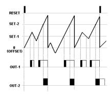
This is the Output-4 state that counting after the set-2 value. OUT-1 output is dependent on OUT-2. TOUT-2 shoul be selected with time. OUT-1 gives an output, the count value rise up to SET-1 value and it stop when it fall down, OUT-2 gives an output when it rise up to SET-2 value, End of the TOUT-2 time outputs and count value is reset automatically. Before the TOUT-2 time is not up, if RESET comes, the outputs and count number are reset.
