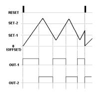
TOUT time sholud be selected as a HOLD. OUT-1 gives an output until the count value reach the SET-2 value and when it reach OUT-1 stop, OUT-2 start to pull. OUT-2 pulls until the count value reach the SET-1 value and when it reach OUT-2 stop and again OUT-1 pulls.
