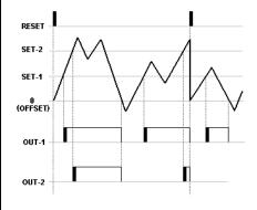
OUT-1 gives an output, the count value rise up to SET-1 value, OUT-2 gives an output when it rise up to SET-2 value and outputs stop end of the TOUT time. If the TOUT times is selected as a HOLD, even count value fall down the SET value, outputs do not stop. When count value reach the zero (OFFSET), the outputs are reset, also when the RESET comes , count value and outputs are reset.
