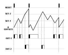
While the count value is under the SET-1 value,OUT-1 gives an output and when rise up, it stop, OUT-2 gives an output when the rise up to SET-2 value, and it stop when fall down the SET-2 value.the count value and outputs are reset when RESET comes.
