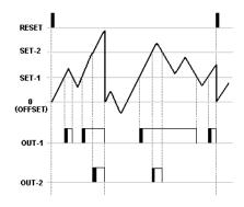
When the count value is over then the Set 1 value,OUT 1 gives an output in this mode (relay-1 pulls). If TOUT-1 (Relay-1 pull time) HOLD is selected, the OUT-1 will be holded up to count value is below SET1. When count value exceed the SET-2 value OUT-2 gives an output and if TOUT-2 HOLD is selected the OUT-2 is holded as a pulled until the count value fall down the SET-2. If TOUT-1 and TOUT-2 is selected with holding time, OUT-1 and OUT-2 will be holded during setted holding time.
