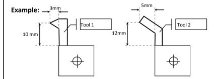
To memory; 2 different tool and to set tool1 as reference and tool2 as selection as left drawing
