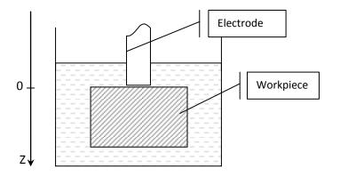
The workpiece wants to be machined up to 50 mm depth as the left side picture. Because of the electrode abrasion the dimension decrease 3 mm. The relay wants to be changed the position when the requested depth is received. To use this EDM function to control the depth; (On X Axis)
