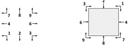
For Tool Diameter Compansation function moves the tool edge to the start point which the machining will be started. And Tan / F3 button is pressed. On work piece the machining side must be selected by numeric buttons. By
