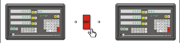
When the work pieces are moved up to make zero all axes you will find the work piece centre.
