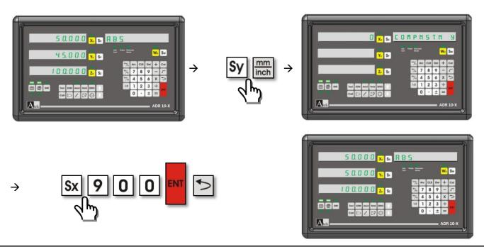
**5.2.2. Segmented Error Compansation Function:** If the scale makes errors in different dimensions this function is used for compensation. It can make compensation up to 100 point. Please select segmented option from system setting menu.
