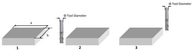
As example the 1st work piece wants to be machined. If you consider only a and b dimensions, because of the tool effect the work piece will be machines wrongly. It is also important which work piece will be machined on which side.
