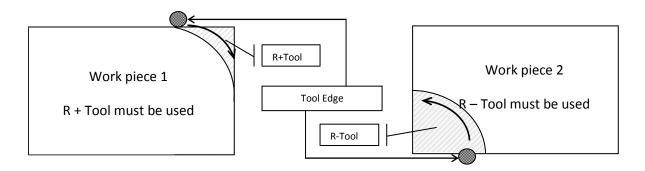
If convex radius will be done as work piece 1 "R+ Tool" must be selected. If the radius will be done concave as work piece 2 "R-Tool" must be selected. Press enter to save.
