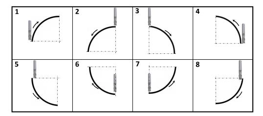
button is used to enter to the function. By button find the "Simple R." writing. Press enter and find the plane by buttons. Press enter to save. On the info screen after "TOOL PATH" writing, select one of the 8 tool ways. After writing the number as 1 to 8 press enter to save. Enter the circle Radius. Press enter to save. Enter "Maximum cutting distance and press enter. Determine if the tool diameter must be add or subtract.
