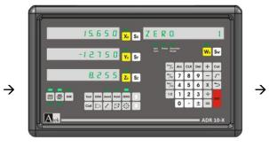
After turning to ABS mode, the changes on X axis are seen on the set coordinate point. In the example 10 mm is added to X axis so 10 mm will be also added to X axis automatically.
