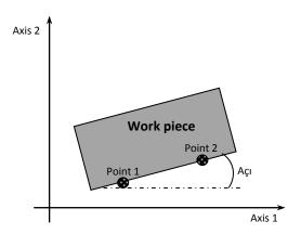
For measuring the tool edge is moved to "Point 1" position. Then press button to enter the function. By buttons select the axes which will be measure and press enter to save. When the tool edge moved to Point 2 on the upper line there is written the angle. On the second line degree.minute.second values are screened by button you can exit.
