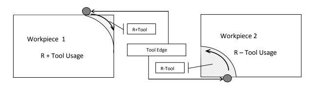
As on the work piece 1 convex would be given R+ Tool should be used. You can travel by button. After selection please press enter to save.
