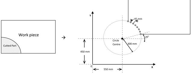
On XY plane, distance of circle centre to X axis is 550 mm, to Y axis is 450 mm, radius is 300 mm, tool diameter 8 mm, max. Cutting distance 45 mm, reference angle 20° finished angle 80° and to applicate smooth radius function:
